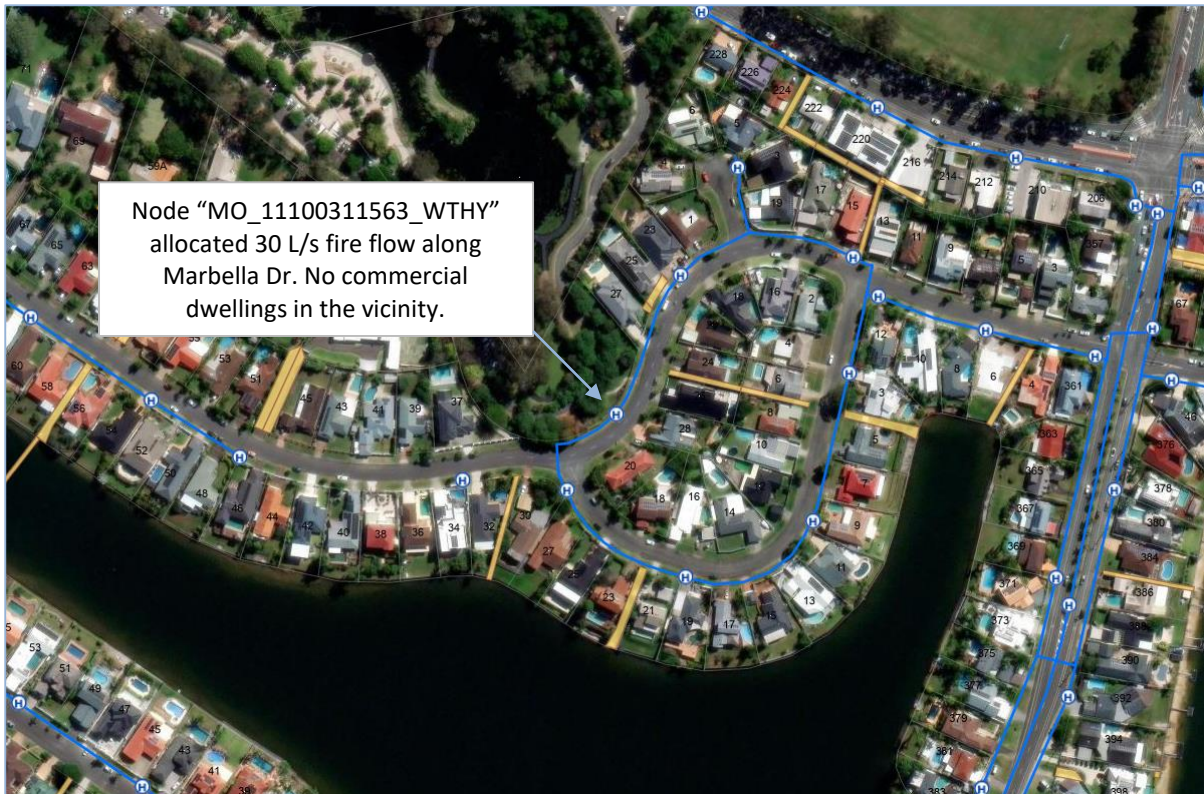
Figure 1. Residential node incorrectly allocated with 30 L/s fire flow (Source: CoGC's online mapping tool)
