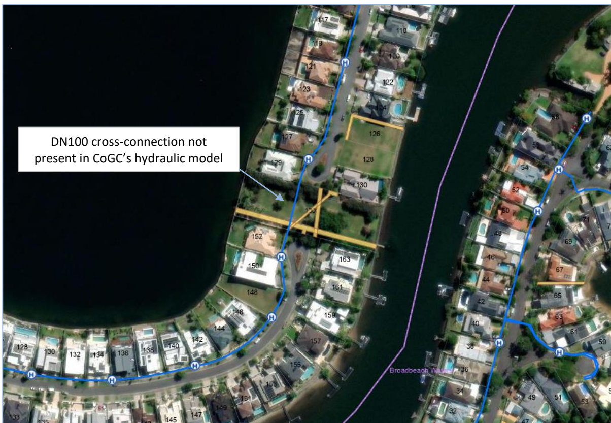
Figure 2. DN100 cross-connection not present in CoGC's model (Source: CoGC's online mapping tool)
